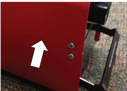
FIGURE 6: SG1000 SEAM ALIGNED
